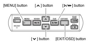
**1** Press the [♥] and [▲] buttons to move the cursor to "REC CONTROL".
